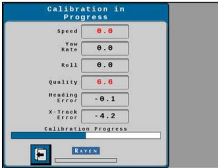
NOTE: Values displayed in red during the calibration process indicate an issue with the calibration parameters and may cause the calibration to stop or require the calibration to be restarted.
