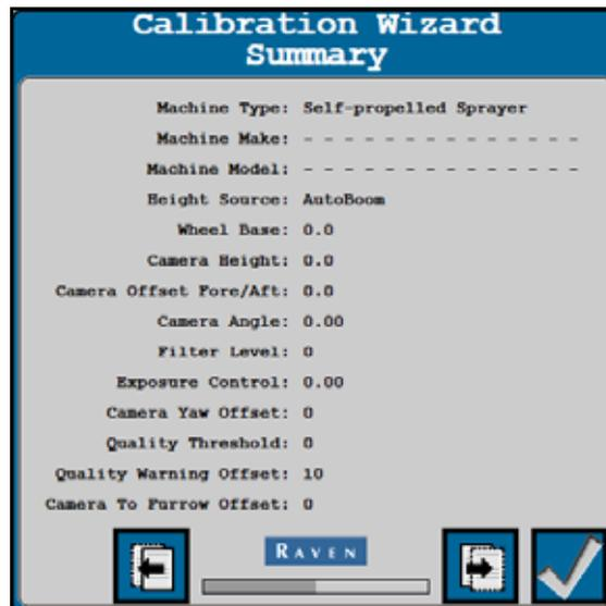
2. To complete the Machine Calibration and save the displayed settings, select the check mark button.
