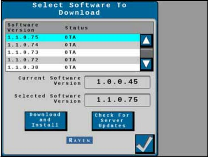
The current software version installed on the VSN system is displayed along with any available OTA (Over the Air) updates.
