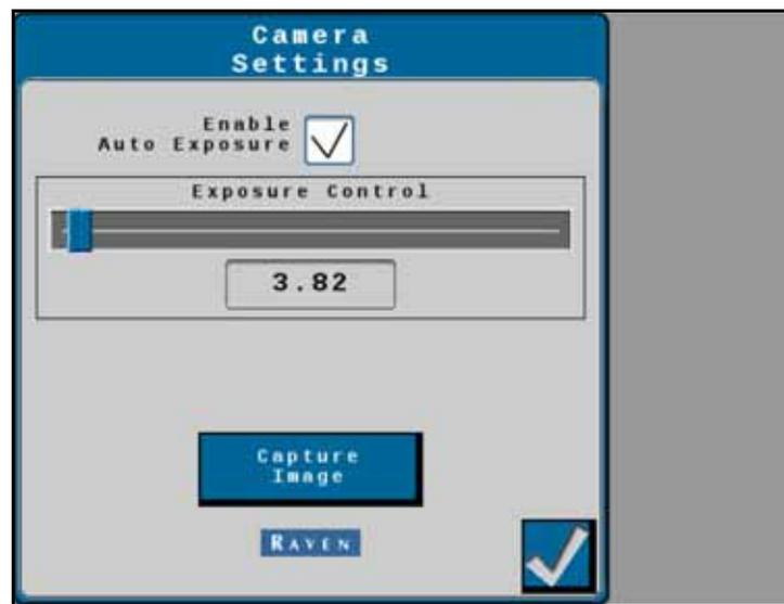
Enable Auto Exposure. Automatically determines the correct exposure for video without any user input. Disable this option to manually adjust camera exposure.
